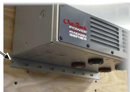
**NOTE:** The left corner is used for securing the inverter to a stud. If the Radian inverter is mounted on plywood or a similar wide-area mounting surface as shown, any of the slots in the mounting flange may be used.
