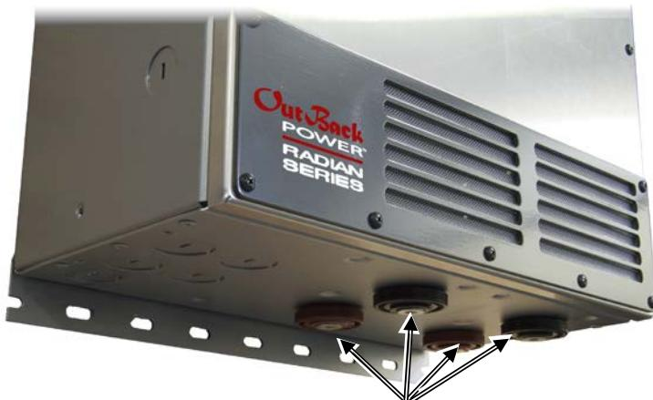
**DC TERMINALS:** Connect to battery cables and DC system. There are two DC positive and two DC negative terminals. Each DC positive terminal requires separate cables and separate overcurrent protection. See page 25 for instructions.
