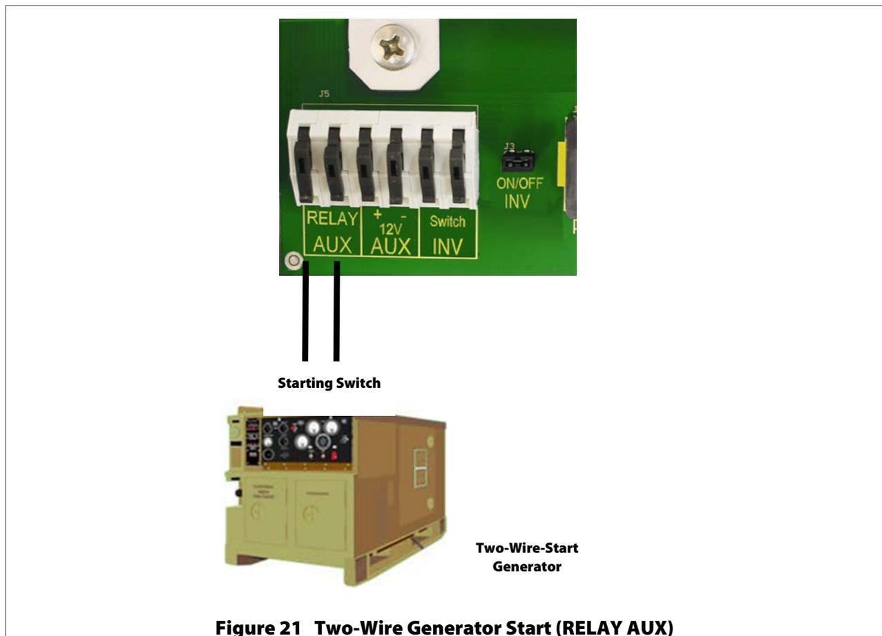
**Figure 21 Two-Wire Generator Start (RELAY AUX)**
